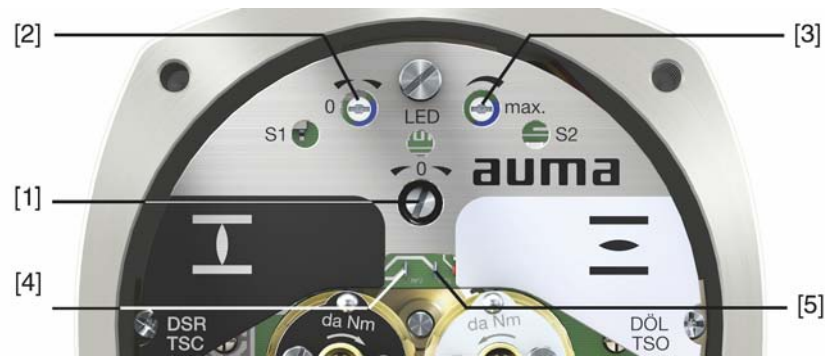
Figure 25: View on control unit when switch compartment is open
