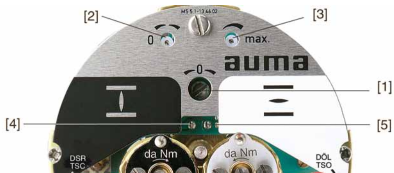
Figure 30: View of control unit
