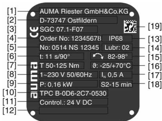
Figure 2: Actuator name plate (example)
