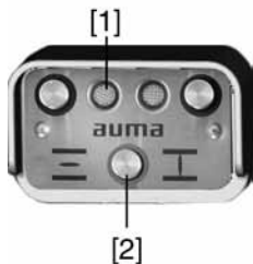
Figure 30: Fault indications and RESET
