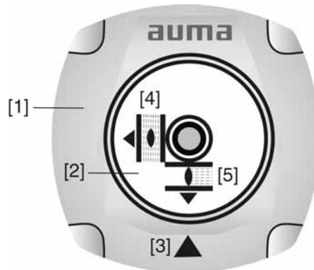
Figure 18: Mechanical position indicator
