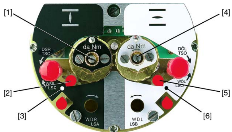
Figure 23: Setting elements for limit switching
