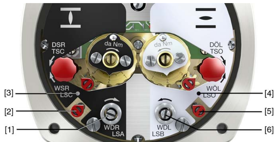
Figure 24: Setting elements for limit switching
